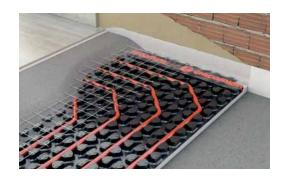
> System for screen-based radiant concrete with smooth panels available in polystyrene foam, polyurethane or eco-friendly materials (wood fiber or cork). The pipes are installed with special locking clips or pipe-fitting rails.
